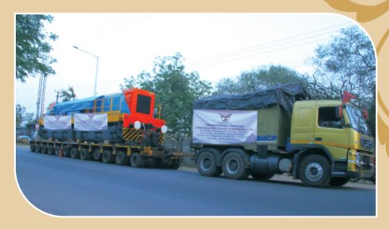
Single Piece, Over Dimensional Consignment weighing approx. 135 MT, with Dimensions 13.5 m x 3 m x 3.45 m, transported from M/s. Ovis Equipments Pvt. Ltd., Cherlapally, Hyderabad (Telangana) to M/s. Penna Cement Industries Ltd., Anantapur (A.P.) in March 2019.
